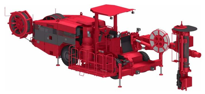
Sandvik DS421 is a rock reinforcement drill rig specialized into cement grouted cablebolts installation in underground mines and tunnels. The Sandvik DS421 is capable of installing up to 25 meters long cable bolts with several steel strands per hole. The drill rig is provided with an on board cement mixer, a cement bags platform and a steel strand reel. It is therefore autonomous for more than a shift.
